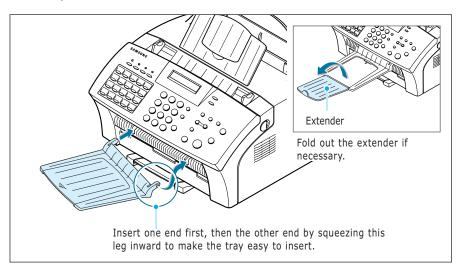
**Note**: The SF-555P is shipped with the paper output tray already installed. Extend the tray to use.
